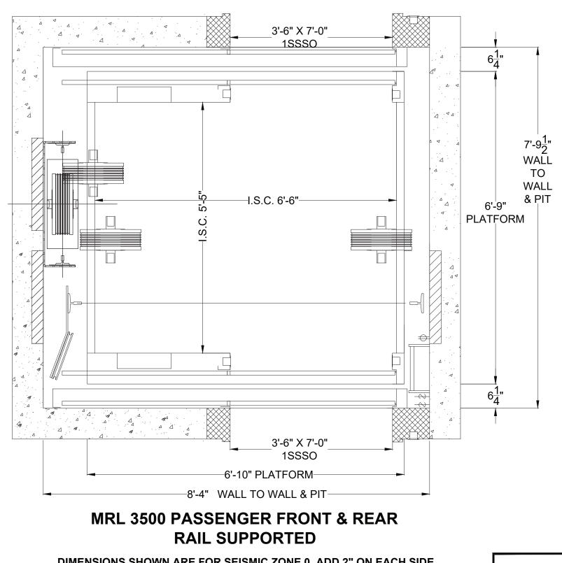
DIMENSIONS SHOWN ARE FOR SEISMIC ZONE 0, ADD 2" ON EACH SIDE **FOR ZONE 2 OR GREATER**
